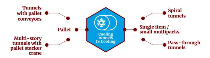
We offer the possibility of chilling a single product immediately after wrapping – in this case we use spiral tunnels and pass-through tunnels with modular belts. Once the product is packed on a pallet, consider using pallet tunnels with pallet conveyors or multi-storey tunnels with pallet stackers.
